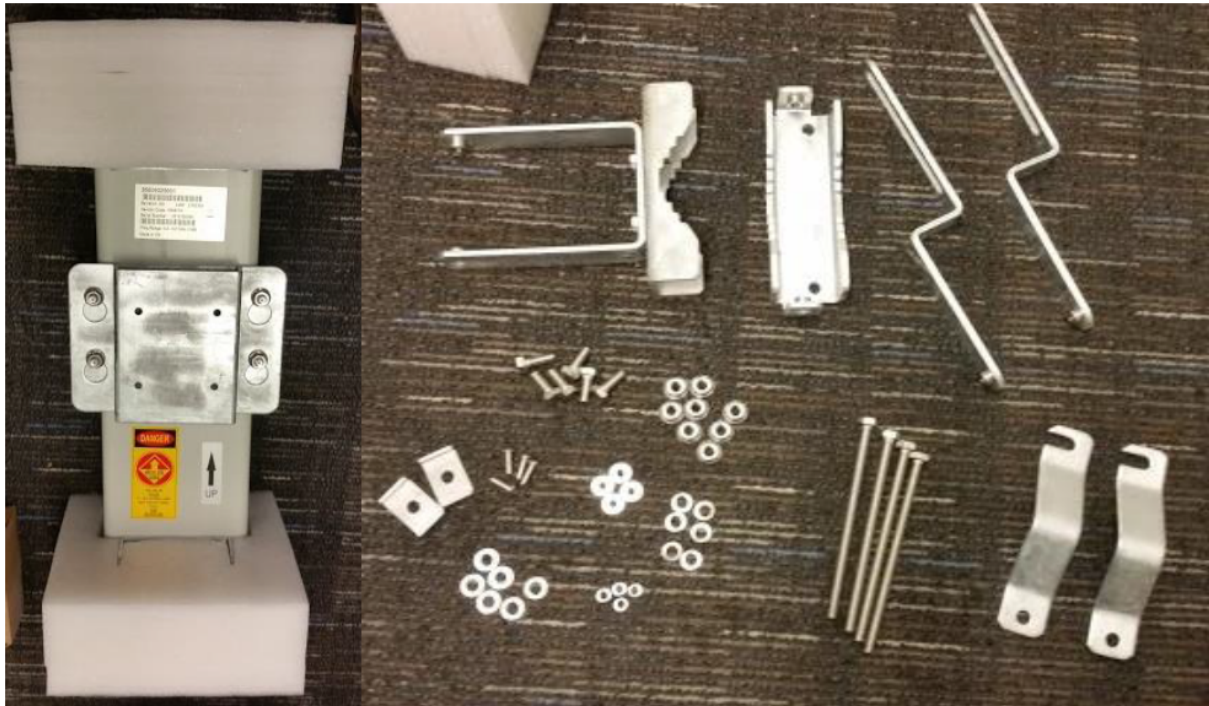
Figure 116: AP antenna parts
