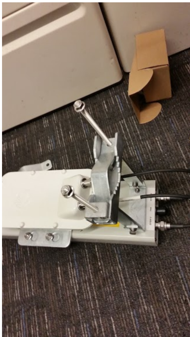
Figure 126: Lower bracket attached to AP antenna
