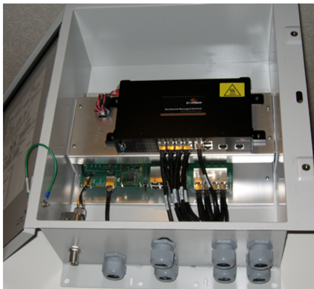
Figure 56: CMM4/CMM5 (Cabinet with switch)
