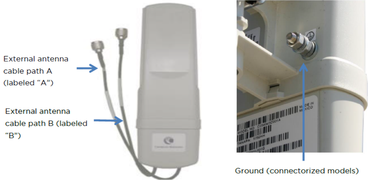
Figure 13 : PMP/PTP 450 Series – SM/BH Connectorized interfaces
