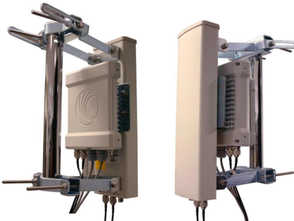
Figure 137: Mounted PMP 450 AP and antenna assembly, viewed from back and back
