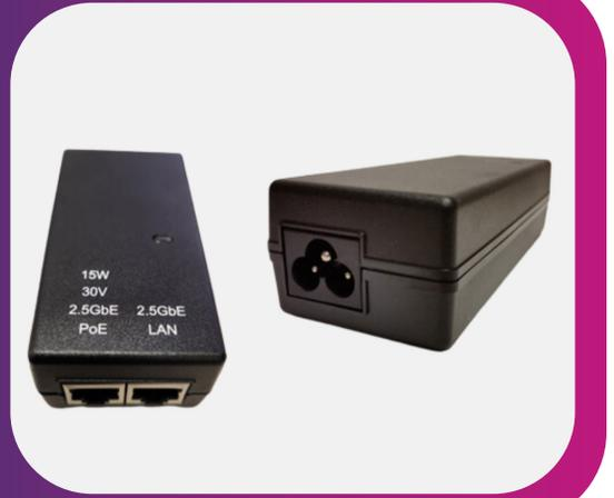
Cambium Networks' radios use PoE (power over Ethernet) for delivering power and data. This PoE power supply has an AC input and a data input, which then drive a 30V power plus data output to the radio. This PoE power supply meets stringent Level VI efficiency requirements and carries regulatory compliance for most locations around the world. The unit is designed to be compact and easy to deploy, while delivering reliability and high performance.
