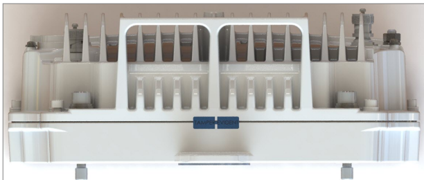
Figure 26: Applying Tamper-Evident FIPS Labels – PTP 850E – Top
