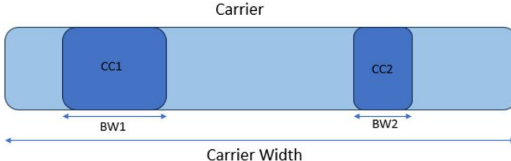
Figure 39: Example of a single carrier with two component carriers
