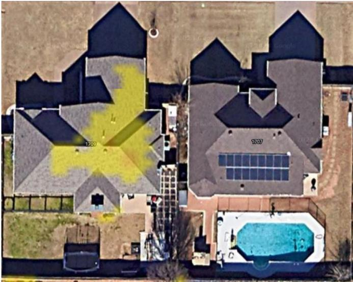
Identify determines home on the left has coverage for the desired install height above the roof and the home on the right does not.
