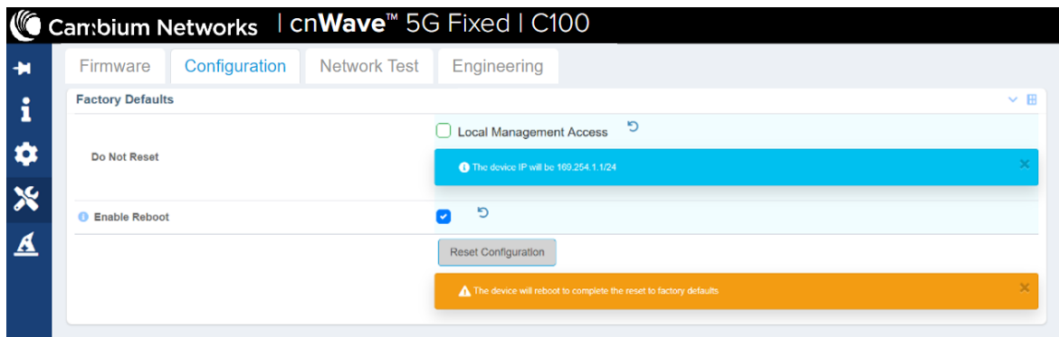
Figure 39: Factory defaults specific CPE parameters
