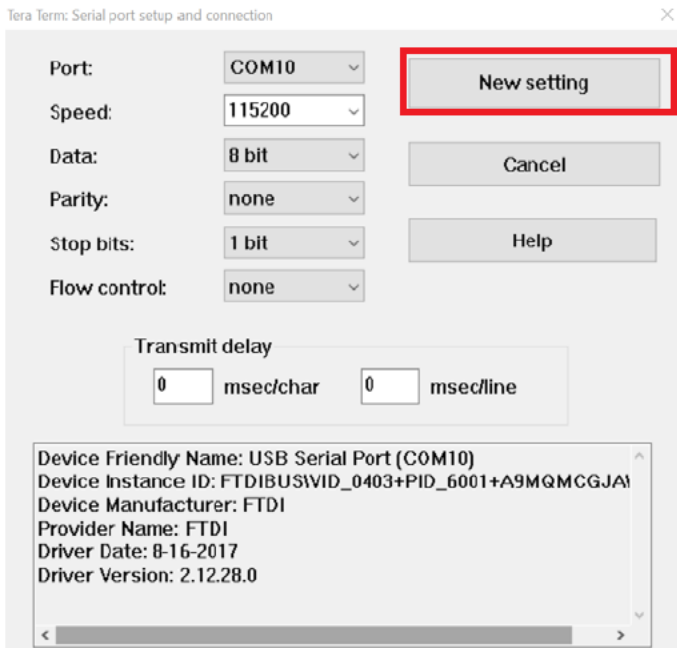
Figure 45: Configuring serial port settings
