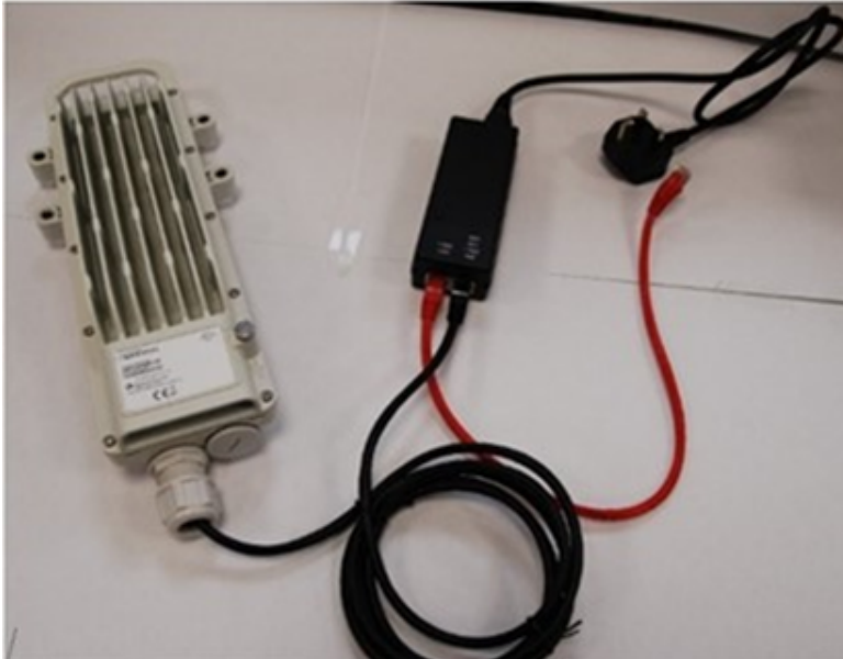
Figure 8: Connecting the CPE to power using a PoE
