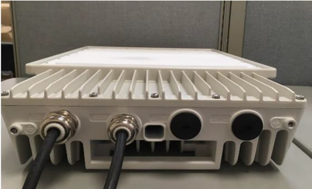
Figure 5: BTS Interface connections
