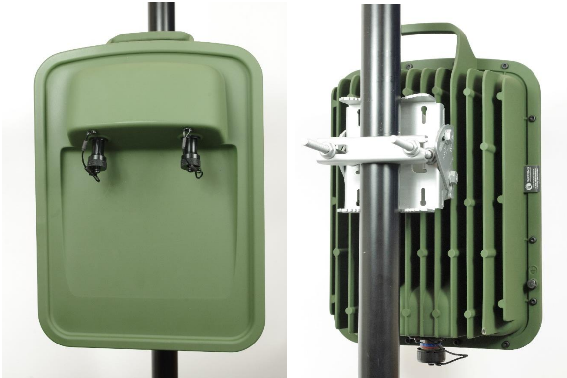
Figure 17 PTP 78700 Connectorized ODU - Green (front and rear views)
