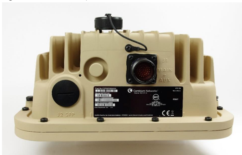
Figure 23 Ethernet and power interfaces for PTP 78700 ODU
