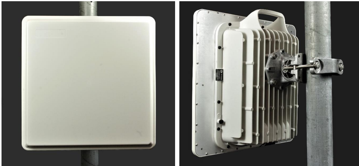
Figure 16 PTP 78700 Integrated ODU - White (front and rear views)
