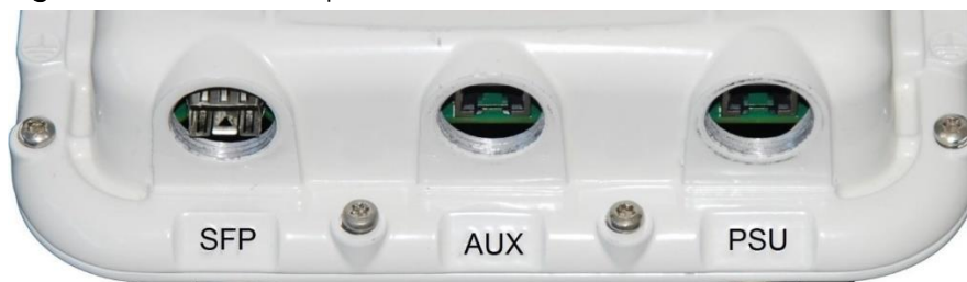
Figure 22 Ethernet and power interfaces for PTP 45700 ODU
