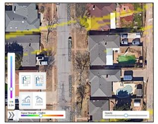
Height and signal strength sliders allow dynamic control of coverage for the heat map.
