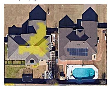
Identify determines home on the left has coverage for the desired install height above the roof and the home on the right does not.
