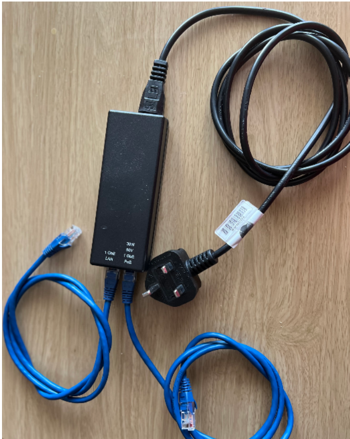
Figure 46 shows how the CPE is connected to the power Injector.
