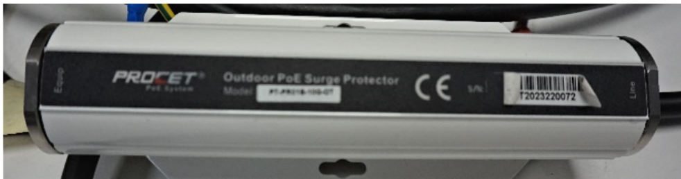
Figure 20: 10G Ethernet LPU - BTS
