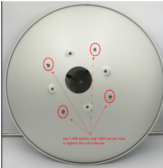
Figure 104: Securing the sub reflector
