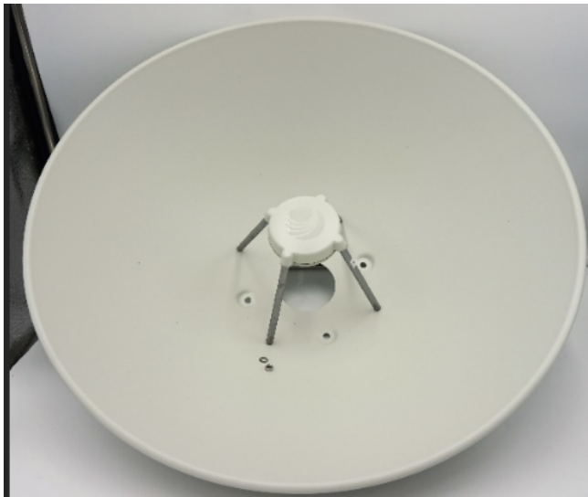
Figure 11: Inserting the sub-reflector
