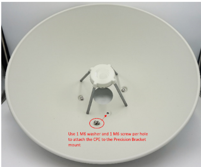
Figure 13: Attaching the dish assembly to the bracket
