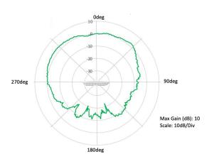
4x4 5 GHz Azimuth
