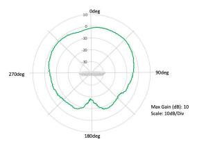
2x2 5 GHz Azimuth
