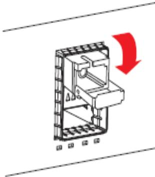
3. Pull the transceiver's out of the slot.
