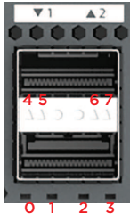
Figure 9: Uplink 3 and 4 LNK and ACT LEDs
