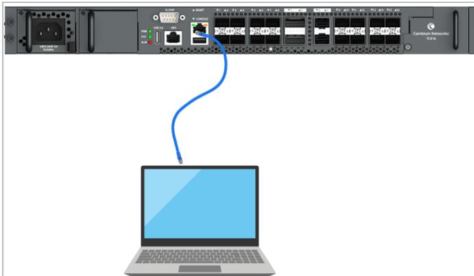
9. Ping *169.254.1.1* to confirm connectivity or open a browser and navigate to *169.254.1.1*, and verify the OLT IP is connected.
