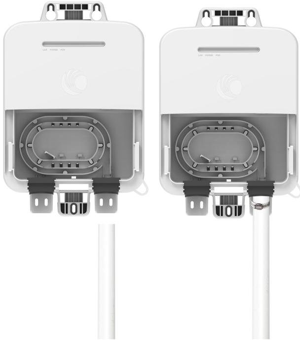
5. Wind the optical fiber cable to the fiber spool, and fix it to the spool with a cable. Then, plug the cable into the PON port.
