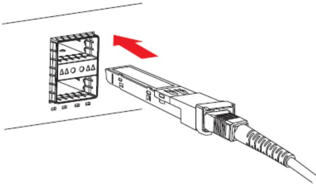
5. Press the transceiver firmly until it fits in its place.
