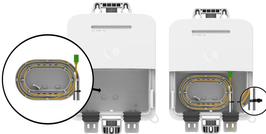
6. Plug in the Ethernet cable to LAN port through the rubber grommet, and fix the cable to the main body with a cable tie.
