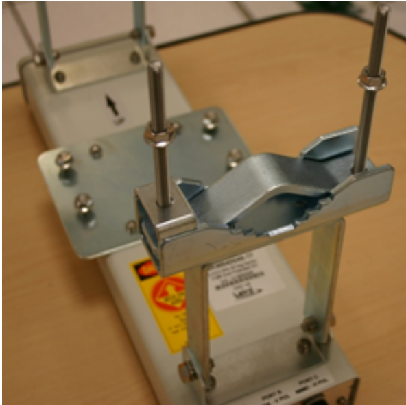
Figure 135: Lower bracket attached to AP antenna
