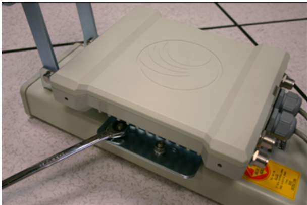
Figure 137: Lower bracket attached to AP antenna
