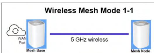
Figure 442 Wireless mesh: 1-1 deployment
